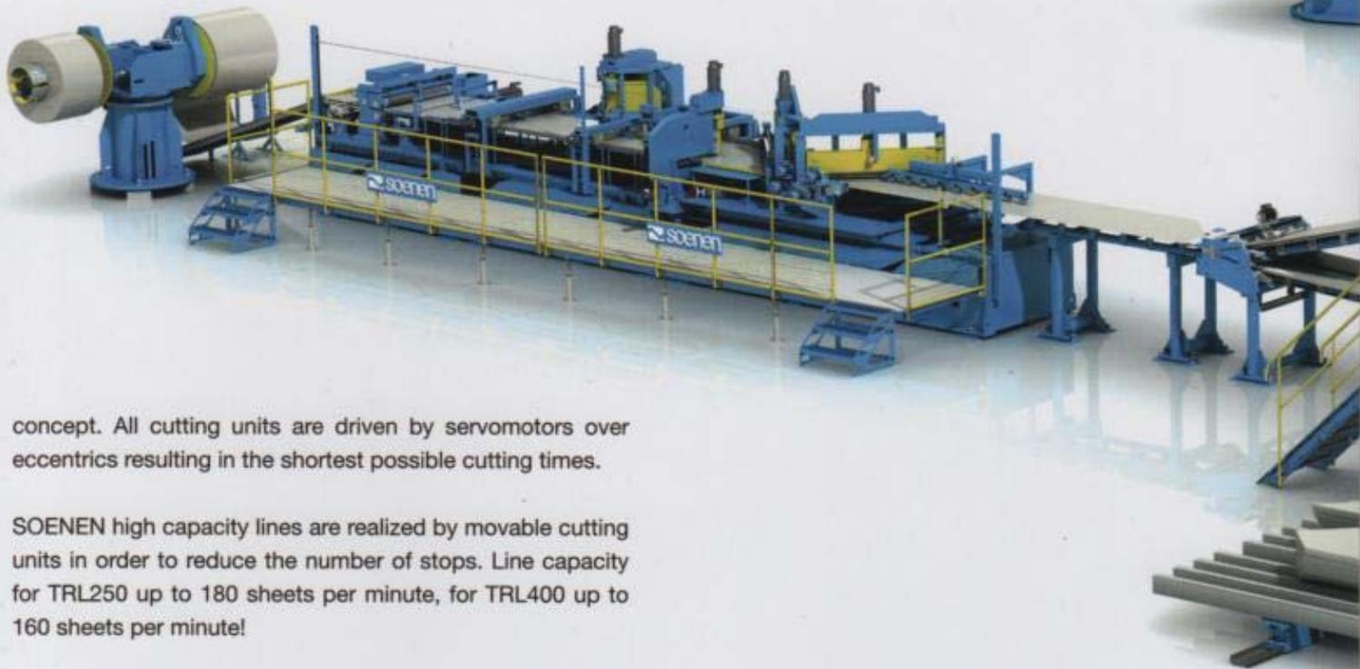
concept. All cutting units are driven by servomotors over eccentrics resulting in the shortest possible cutting times.
