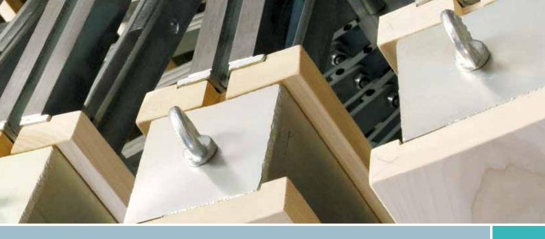
a right and a left one. The steel beams are assembled on running guides operated by the running support by means of levers which make the cylindrical shapes appear. The wood covering allows the final work to be done, thus obtaining the perfect cylindrical shape of expanding equipment.
