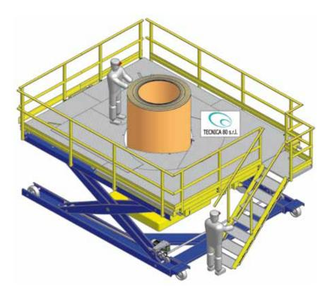
The plan is itself divided into two opening parts for the introduction of the bobbin in the centre of the platform. The platform is equipped with a scale for operator access and is equipped with adjustable steps with landing for entrance to the platform, and a security perimeter railing along the top edge of the platform.
